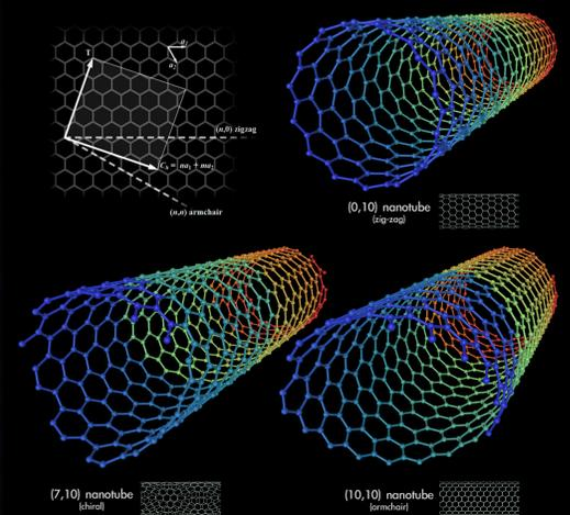
Different Types of Carbon Nanotube Structure
